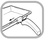
Slide the handle towards the centre of the pan and let the handle locate over the bracket.
